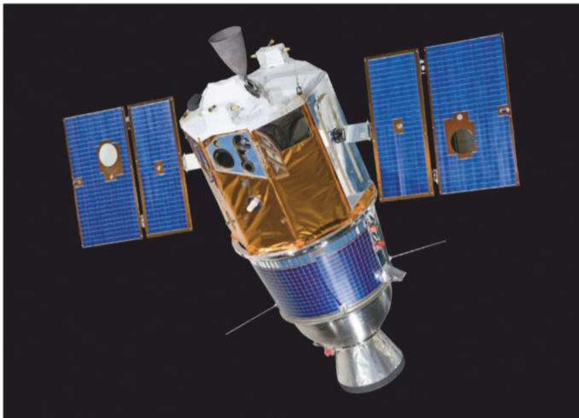
**Above: Lidar measurements of lunar topography from the Clementine mission. Left: The Clementine model; its interstage and solid rocket motor (bottom half) were discarded before insertion into lunar orbit.**
