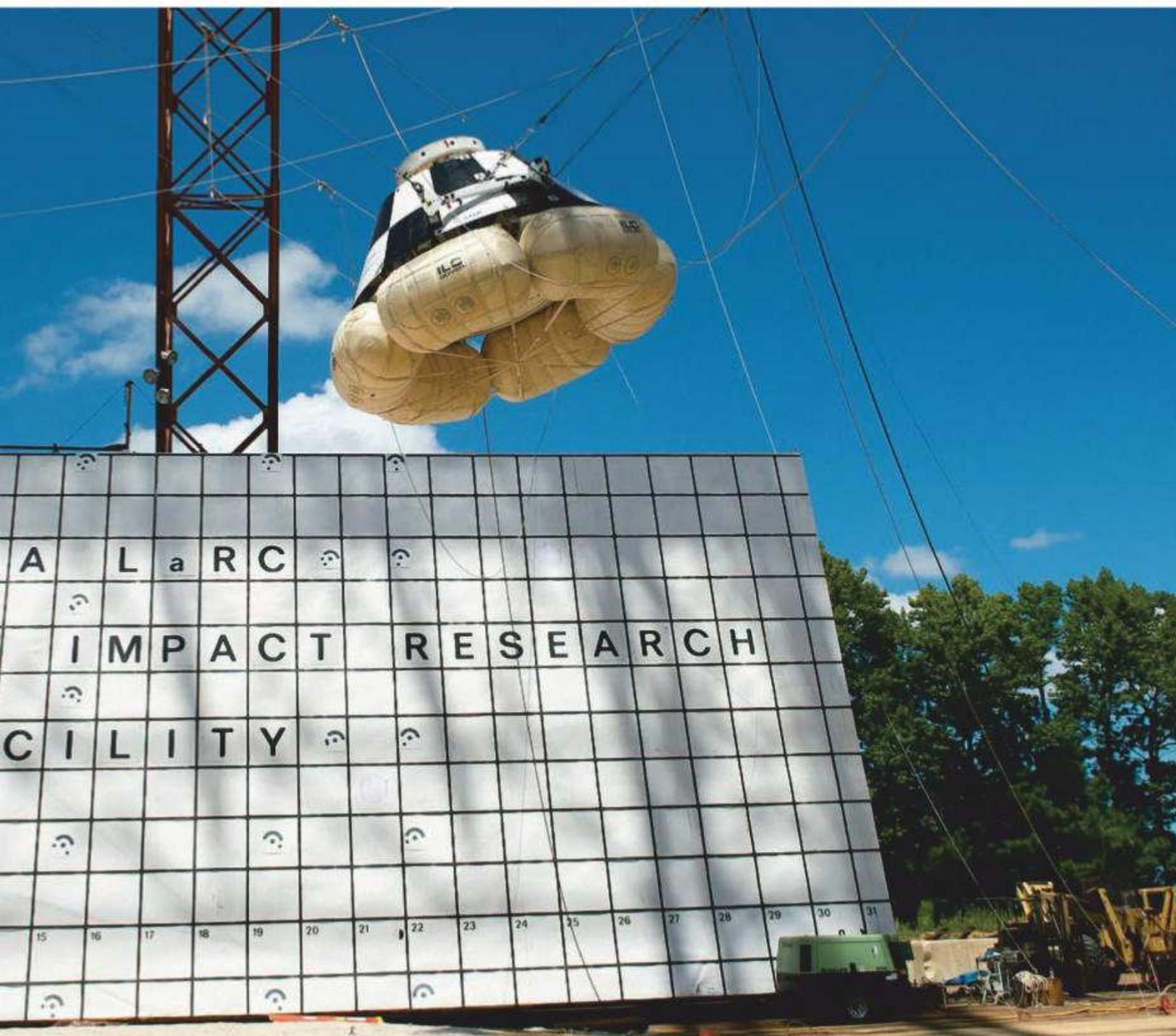
**Instead of the Soyuz’s heavy retrothrusters, Boeing designed six lightweight airbags for the Starliner (being tested at Langley Research Center, left) that should put a somewhat more comfortable bounce in its drop back to Earth.**
