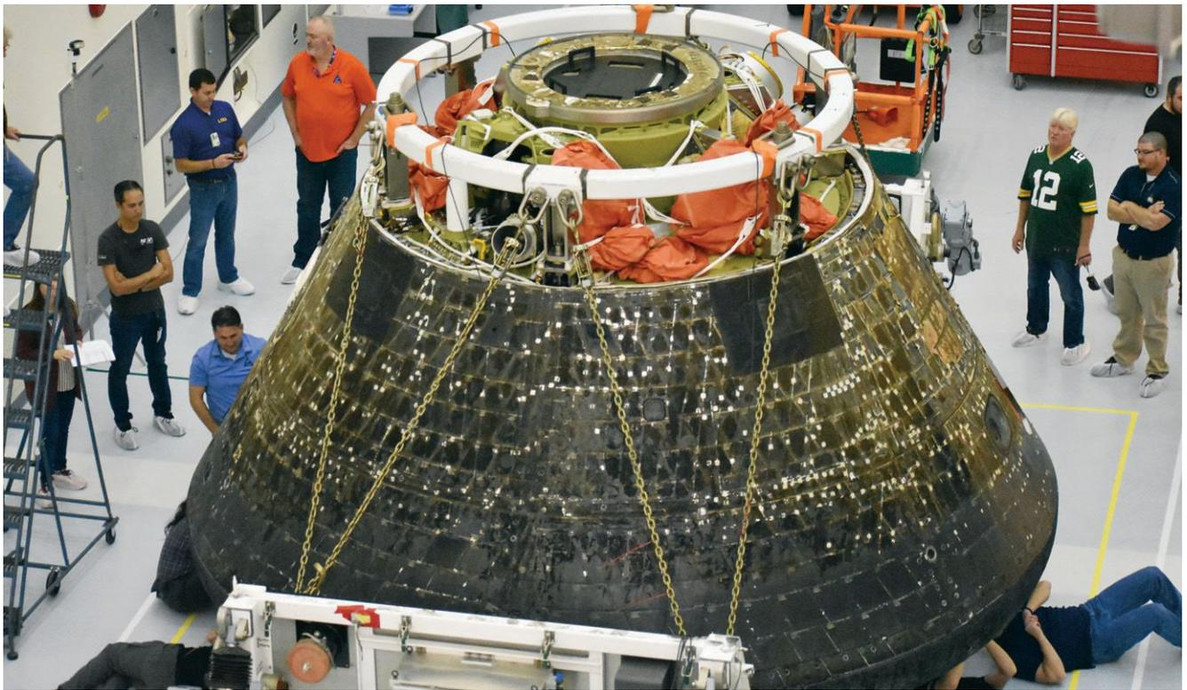
▲ NASA is still analyzing the heat shield of the Orion capsule that completed the Artemis I flight. More material eroded during atmospheric entry than expected, prompting the agency to push back the crewed Artemis II mission to September 2025, a delay of one year.
