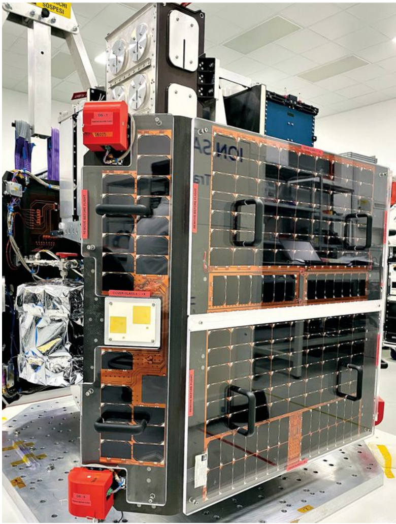
▲ D-Orbit's fifth ION Satellite Carrier at the company's Italy headquarters before its April launch aboard a SpaceX Falcon 9. Two of the customer satellites can be seen peeking over the top of the black solar panels that encase the cube-shaped dispenser. The silver box at left covers ION's propulsion tanks, and the red boxes cover multisensor modules.
