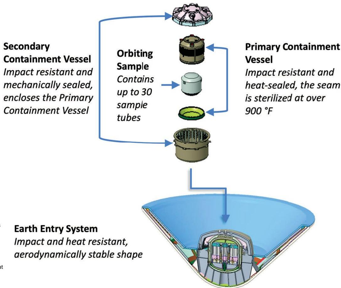
► This graphic showed during one of NASA's public briefings on the environmental risks of Mars Sample Return illustrates how the samples would be ensconced inside two vessels within the Earth Entry System spacecraft that would return them to Earth.
