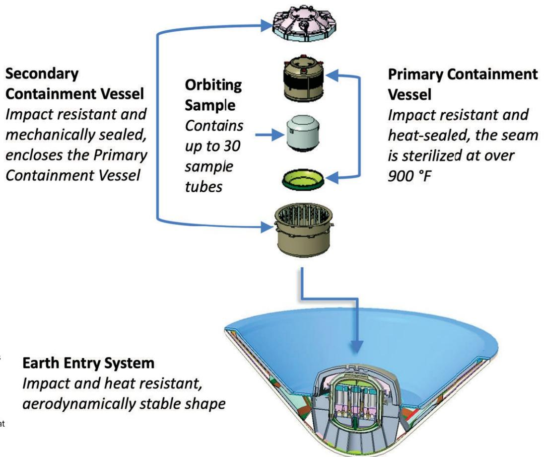
► This graphic showed during one of NASA's public briefings on the environmental risks of Mars Sample Return illustrates how the samples would be ensconced inside two vessels within the Earth Entry System spacecraft that would return them to Earth.
