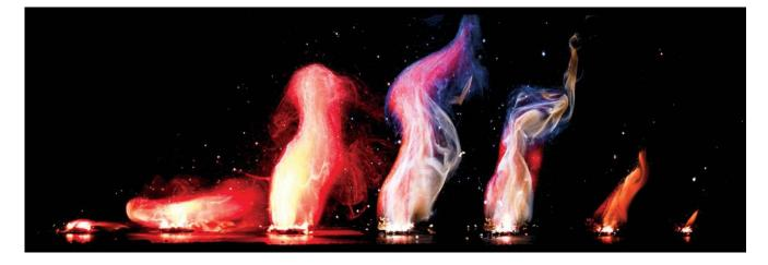
▲ Purdue University students tested a mix of 60% calcium perchlorate and 40% magnesium perchlorate to simulate how a solid propellant created from Martian soil might burn. As shown in this time-lapse image, their "Mars propellant" created red, white and blue flames. Purdue University
