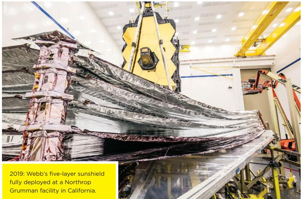
2019: Webb's five-layer sunshield fully deployed at a Northrop Grumman facility in California.
