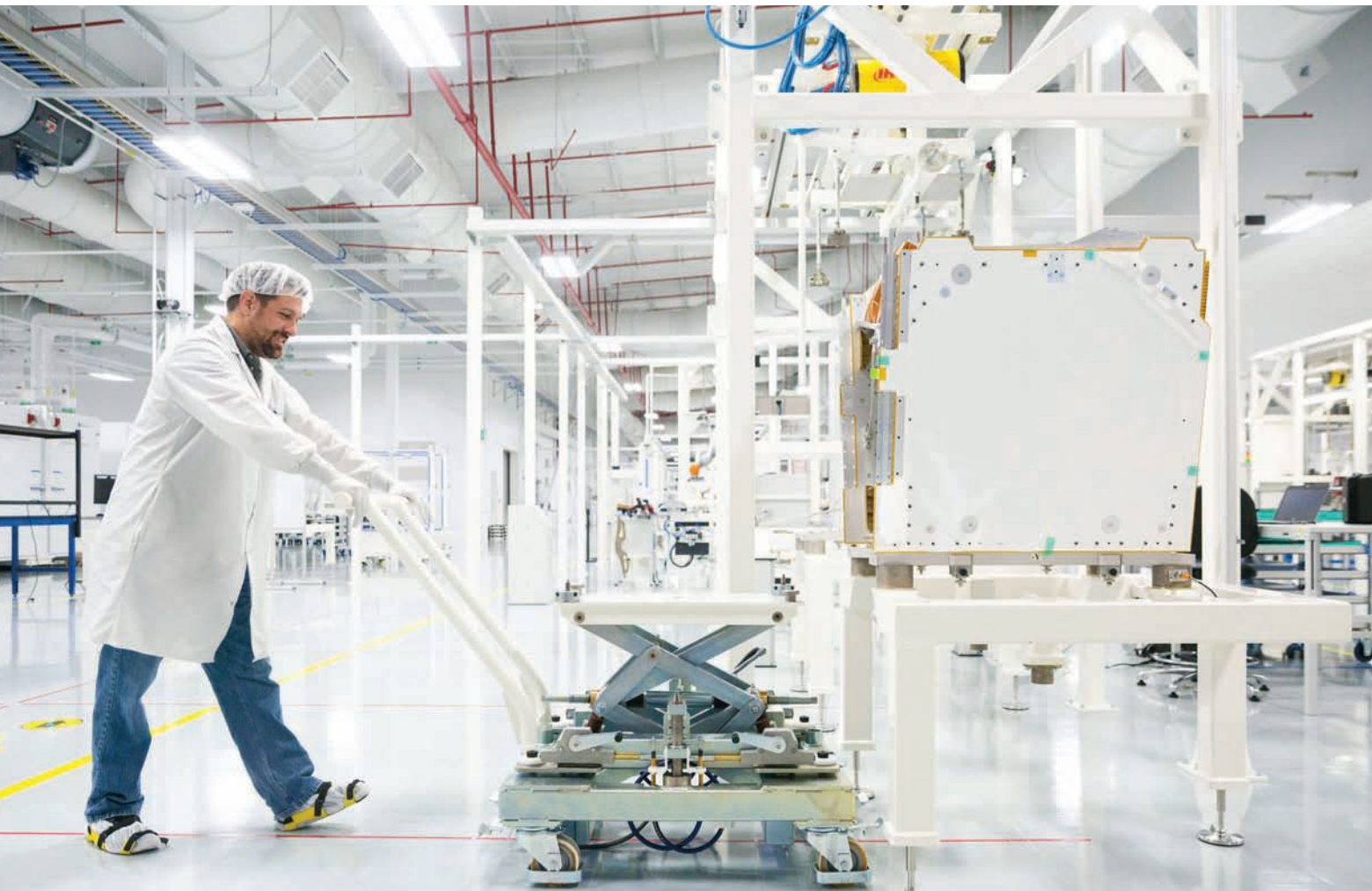
▼ An engineer prepares to move a completed OneWeb satellite to a chamber to test for extreme temperatures. OneWeb Satellites
