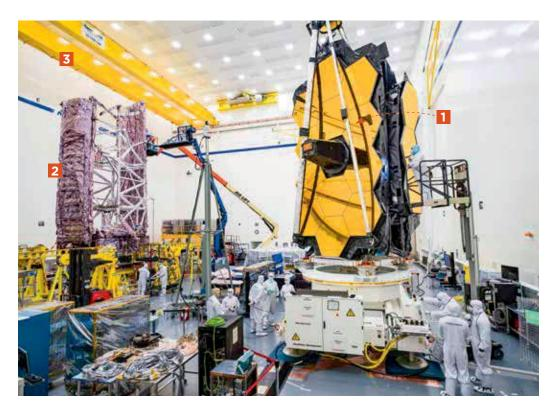
o this point, NASA and Northrop Grumman have steered the massive James Webb Space Telescope through development in two halves. Engineers had to do that, partly because in space the two halves must function at opposite temperature extremes. No facility could replicate near absolute zero on one side of the spacecraft and sunlight on the other.
