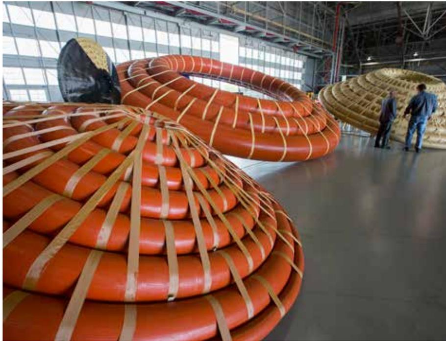
ifornia. Engineers pumped compressed water into the doughnutlike tubes while they were submerged in a pool of water to test how much pressure they could withstand.
