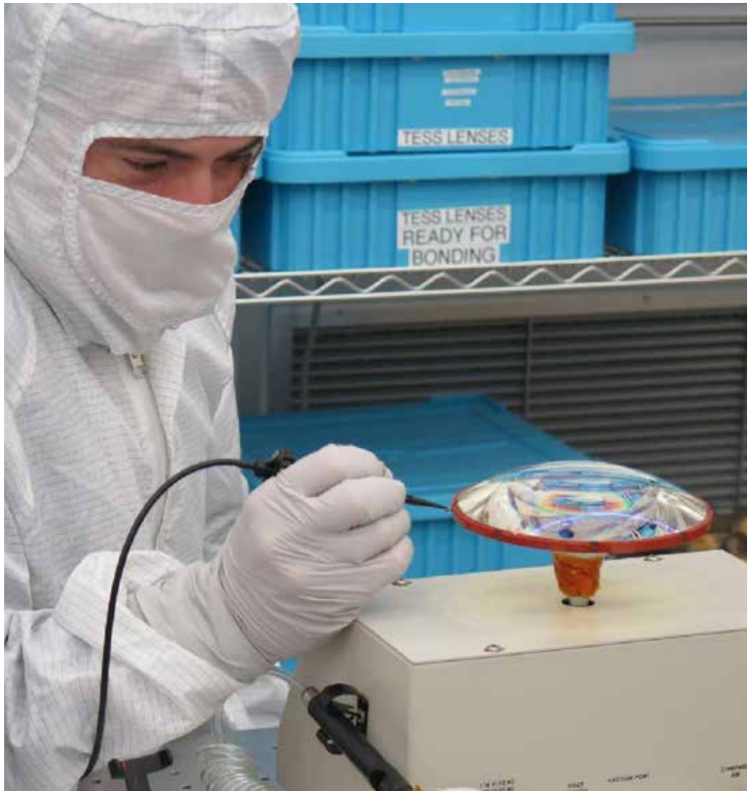
An optical engineer at MIT Lincoln Laboratory applies room-temperature vulcanizing silicone to a TESS flight lens. A complication with the RTV caused some concern during testing. MIT Lincoln Laboratory
