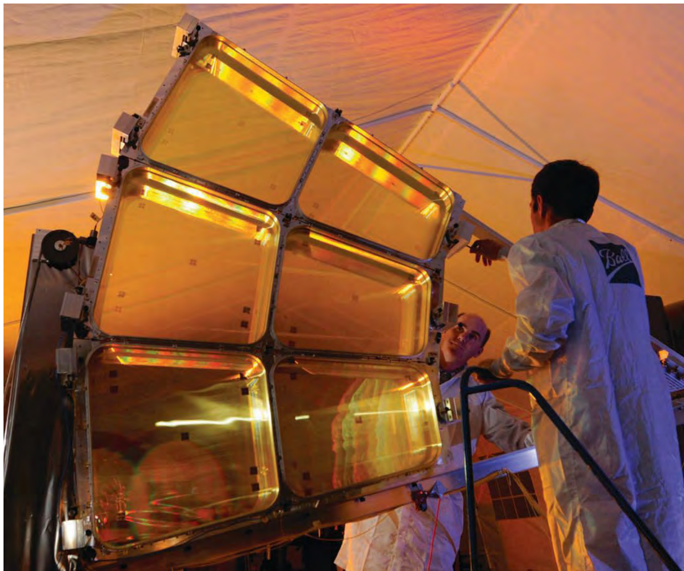
For a test of lightweight optical technology, Ball Aerospace engineers erected a set of six 20-micron-thick diffractive optical elements on a frame to represent one-eighth of a 5-meter-diameter membrane telescope.
