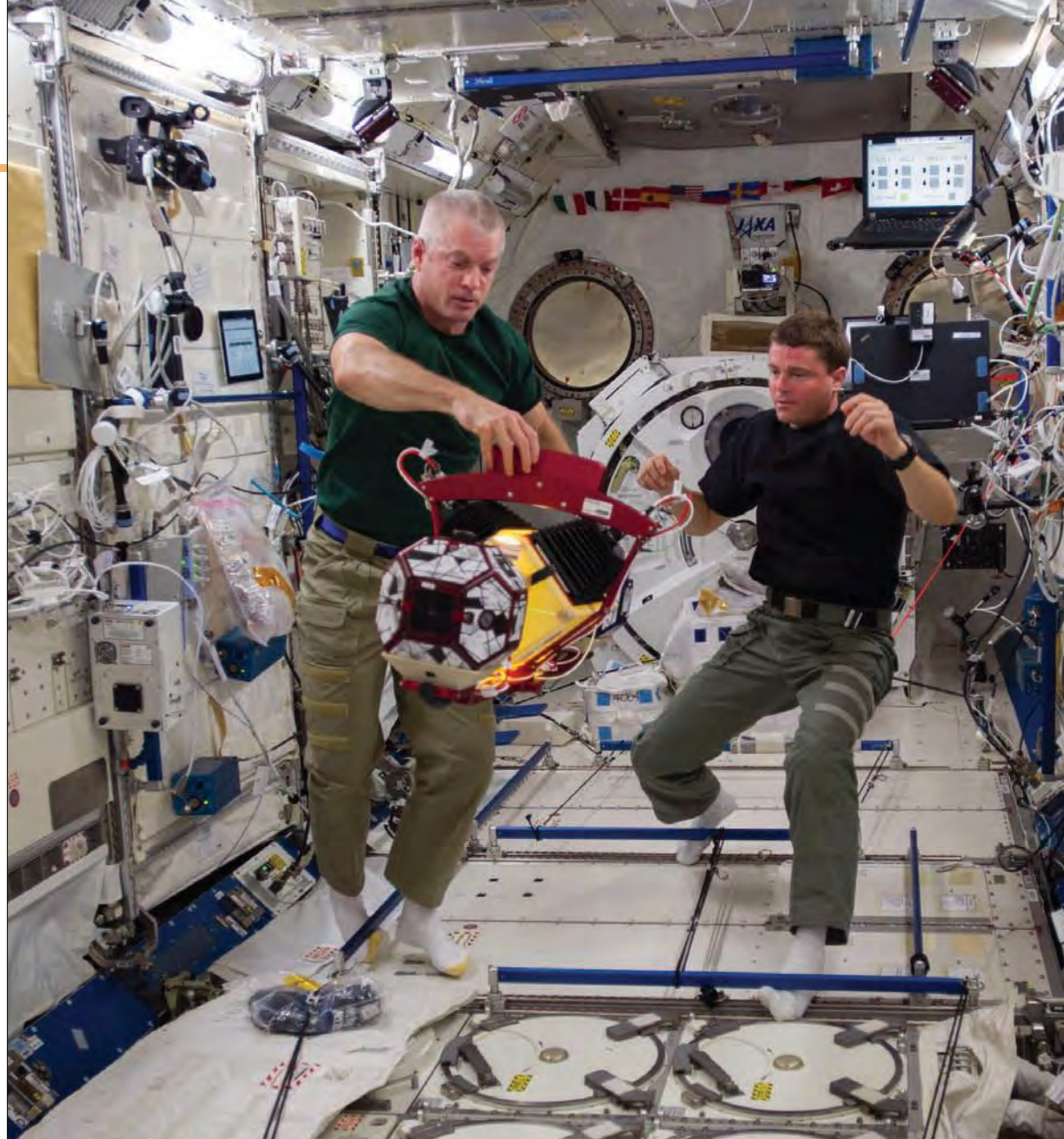
Steve Swanson, left, and Reid Wiseman conduct test runs of the SPHERES-Slosh experiment, which uses soccer-ball-sized Synchronized Position Hold, Engage, Reorient, Experimental Satellites to examine how liquids move inside containers in microgravity.
