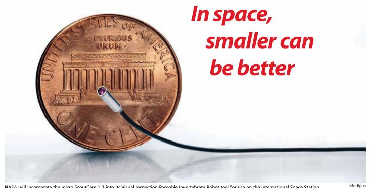
NASA will incorporate the micro ScoutCam 1.2 into its Visual Inspection Poseable Invertebrate Robot tool for use on the International Space Station.
