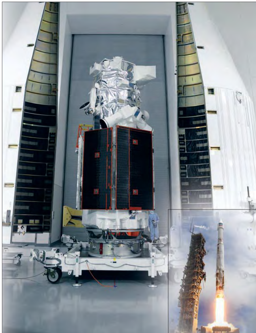
The WorldView-3 satellite is encapsulated within the Atlas 5 rocket. Its August launch came shortly after relaxation of government restrictions on satellite imagery for commercial customers.
