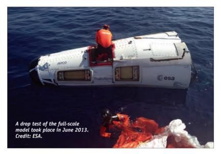
This marked the genesis of the Intermediate Experimental Vehicle, initiated as part of ESA's Future Launcher Preparatory Program in 2004. According to Quaglino, following "a thorough industrial trade-off on shape and system concepts...the concept selected for the IXV was a lifting re-entry body," designed for launch by ESA's Vega rocket on an equatorial trajectory leading to re-entry and parachute-assisted splashdown in the Pacific Ocean about 100 minutes later.
