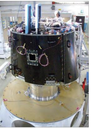
The rear segment of the Intermediate Experimental Vehicle on an integration stand. Credit: ESA/Thales Alenia Space. The potential advantage for European countries lies in their penchant for applying technology to commercial applications – in the satellite manufacturing and launch industries, for example. That ESA is funding a re-entry demonstrator suggests the potential for future commercial application.
