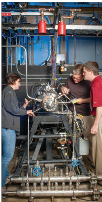
Task lead Tyler Hickman, in red shirt, and technicians inspect the additively manufactured rocket injector assembly as it is installed in the Rocket Combustion Laboratory at NASA Glenn. Courtesy NASA.
