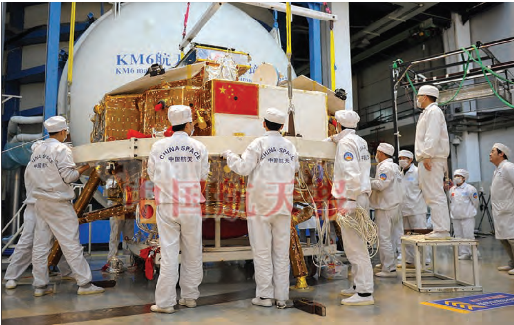
Technicians show the overall scale of the Chinese lander and the boxy design similar to the Apollo lunar module. But unlike Apollo, the plutonium 238 RTG-powered Chinese lander is to survive for an Earth year and carries science instruments including a drill and telescope. Rover is designed to drive up to 6 mi. during three Earth months of operation. Credit: China Space News/NASASpaceflight.com/Planetary Society.
