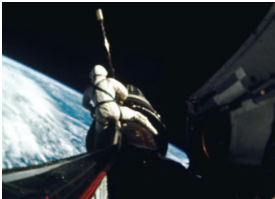
Gemini XI astronaut Dick Gordon straddles the Agena spacecraft docking collar during his second EVA, on Sept. 13, 1966. Gordon struggled to complete his spacewalking tasks because of insufficient handholds and tethers outside, a problem finally resolved on Gemini XII. Courtesy: NASA.
