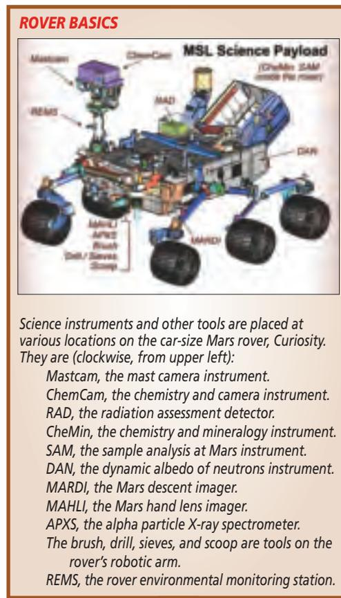
Science instruments and other tools are placed at various locations on the car-size Mars rover, Curiosity. They are (clockwise, from upper left):
