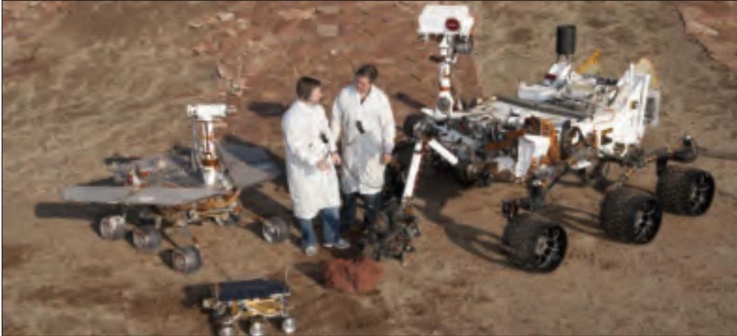
*Spacecraft engineers stand with three generations of Mars rovers developed at JPL: Front and center is the Sojourner flight spare; at left is a rover akin to Spirit and Opportunity; to its right is a Curiosity-size test rover. Credit: NASA/JPL-Caltech.*
