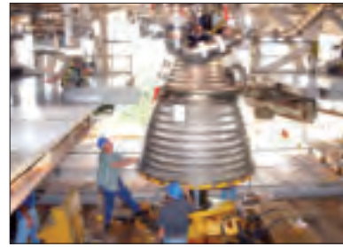
A highly uprated and modernized version of the Pratt & Whitney Rocketdyne J-2X used originally in the Apollo second and third stages will be the upper-stage engine Block 1 SLS. It will have 294,000 lb thrust, 69,000 lb more than the Apollo J-2. NASA Image.
