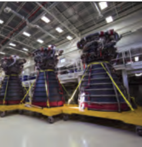
The six space shuttle main engines (SSMEs) that powered Endeavour and Atlantis on the final two shuttle missions are readied at KSC for shipment to Pratt & Whitney Rocketdyne. There they will be prepared for use as expendable engines on early SLS flights. NASA image.
