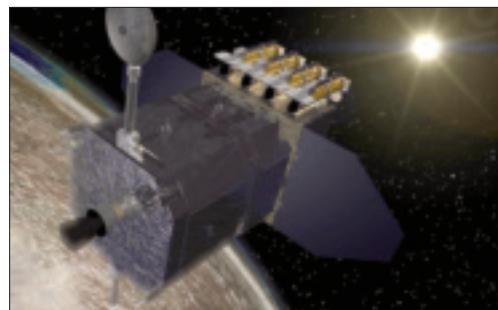
Equipped with the most powerful civilian data system ever flown, the \$850-million SDO is studying the solar atmosphere on small scales of space and time and in numerous wavelengths simultaneously. It is the highest resolution solar spacecraft ever launched.
