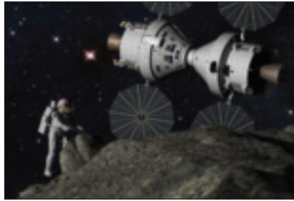
Lockheed Martin's Plymouth Rock mission concept would use a pair of Orion spacecraft to take an astronaut crew to a nearby asteroid. The vehicle would support a crew for about 6 months, including a two-week exploration phase at the asteroid. Image courtesy Lockheed Martin.
