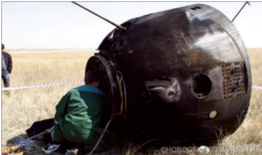
Heat damage is evident on the Soyuz TMA-11 descent module after landing on April 19, 2008. Astronauts will have to respond to similar in-flight emergencies in the era of ISS, Soyuz, and commercial crew spacecraft. (Photo: Novosti/Aleksandr Pantyukhin)
