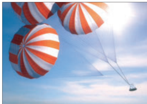
The Dragon drop test validated the parachute deployment system.
