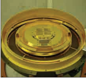
IBEX has two sensors, IBEX Hi (seen here) and IBEX Lo. Each time an energetic neutral atom comes into one of the sensors, it is recorded; at the end of six months of that data scientists will have a picture of the entire 360° longitude celestial sphere. (Photo courtesy Southwest Research Institute.)
