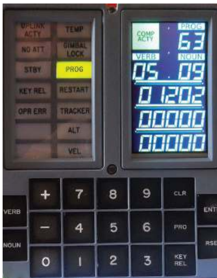
What the 1202 computer alarm looked like to Armstrong and Aldrin aboard the Lunar Module. This is a modern reproduction of the Apollo Guidance Computer. Credit: Nick Howes
