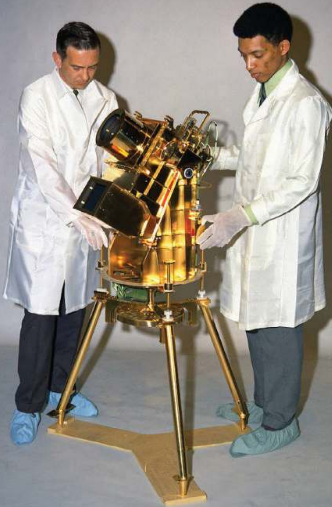
Dr. George Carruthers, right, and William Conway, a project manager at the Naval Research Institute, examine the gold-plated ultraviolet camera/spectrograph, the Moon-based observatory that Carruthers developed for use on the Apollo 16 mission.
