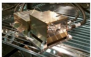
Figure 4: Chang'E4 LND flight model sensor head (front) and EBox (back) before their thermal tests.
