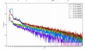
Fig. 3: Calibration results for thermal neutrons. The two small peaks indicated by the arrows are due to thermal neutrons.
