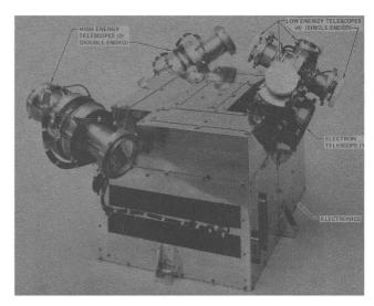
mass, and direction of each entering particle is measured by the number of detectors it penetrates, the electrical charge it deposits, and which telescope it enters. The telescopes are positioned at various angles to that the experiment does not need spacecraft maneuvers to gather samples from all directions.
