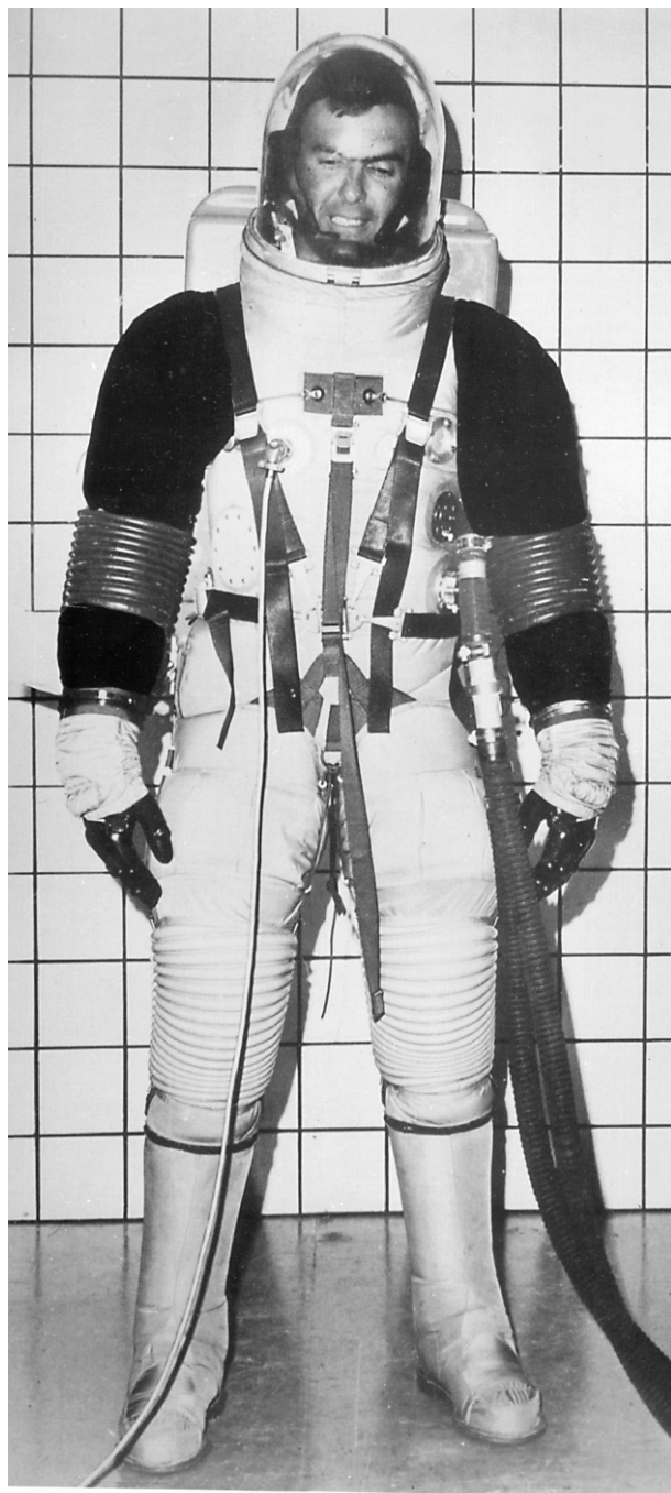
Figure 6.5.7. ILC rear-entry SOA suit with “blacked out” shoulders (courtesy ILC Dover LP).
