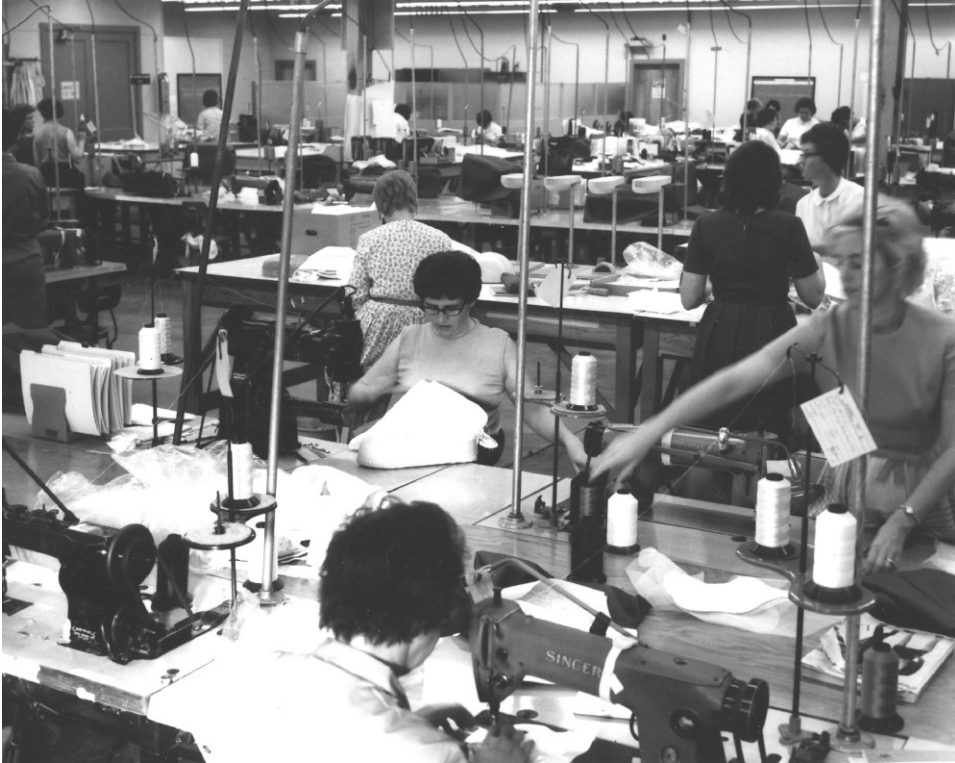
Figure 6.7.3. A7L suit production floor at International Latex (courtesy ILC Dover LP).
