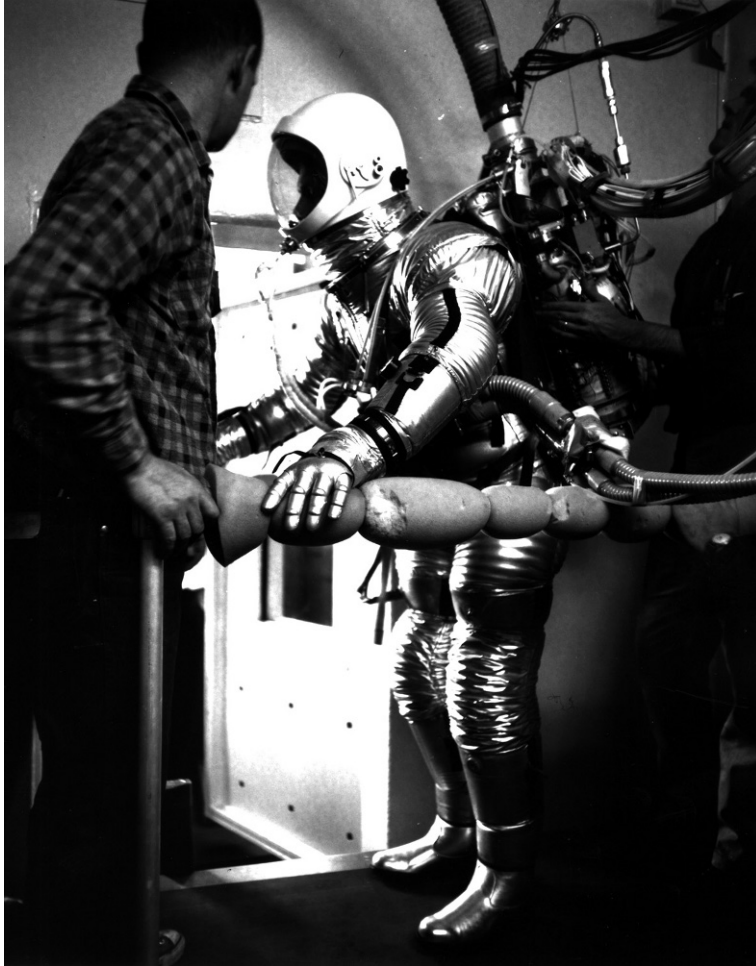
Figure 6.2.7. First AX1H suit and life support testing (courtesy Hamilton Sundstrand).
