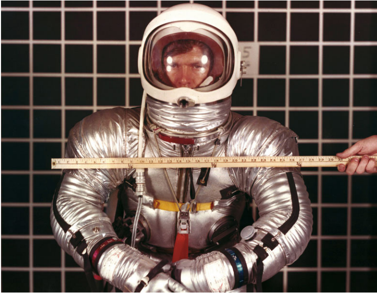
Figure 6.2.6. AX1H-021 shoulder width measurement (courtesy Hamilton Sundstrand, Windsor Locks, CT).
