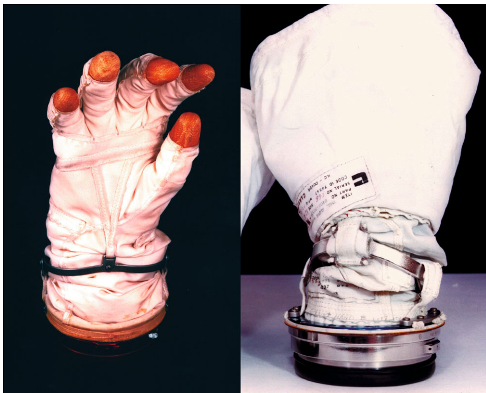
Figure 10.1.13. Original and production 1000 series glove (courtesy Hamilton Sundstrand).
