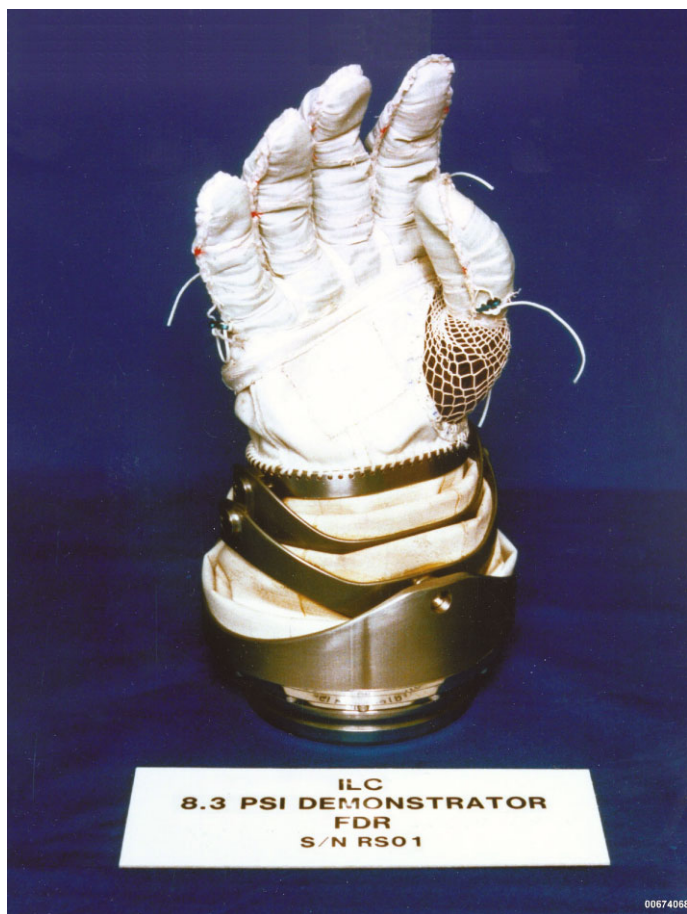
Figure 11.1.13. ILC's Mark III, 8.3 psi glove (courtesy Hamilton Sundstrand).
