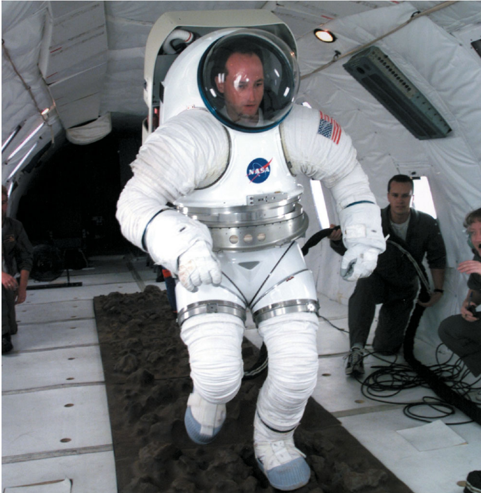
Figure 11.3.10. H-suit in lunar/Mars gravity walking tests (courtesy NASA).
