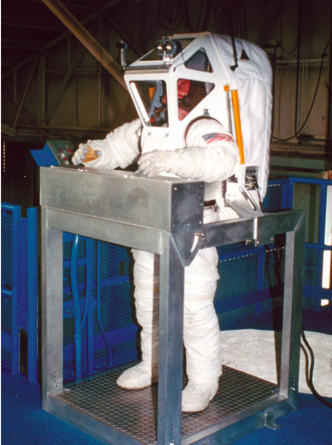
Figure 11.3.3. 1990 Griffin command/control pressure suit upper-torso prototype (courtesy G. L. Harris/B. Griffin).
