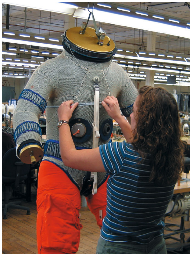
Figure 4.7.3. ACES upper-torso Link-net restraint system (courtesy David Clark Co.).
