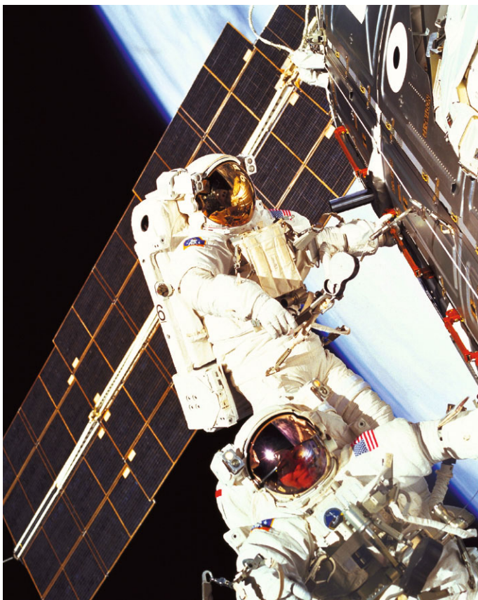
Figure 10.2.11. STS-88 baseline (foreground) and enhanced EMUs assembling the ISS (courtesy NASA).
