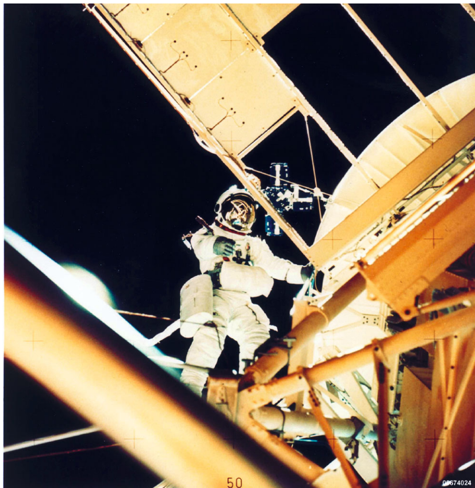
Figure 9.3.7. SOP shown on Owen Garriott's EMU during a Skylab 3 EVA (courtesy NASA).
