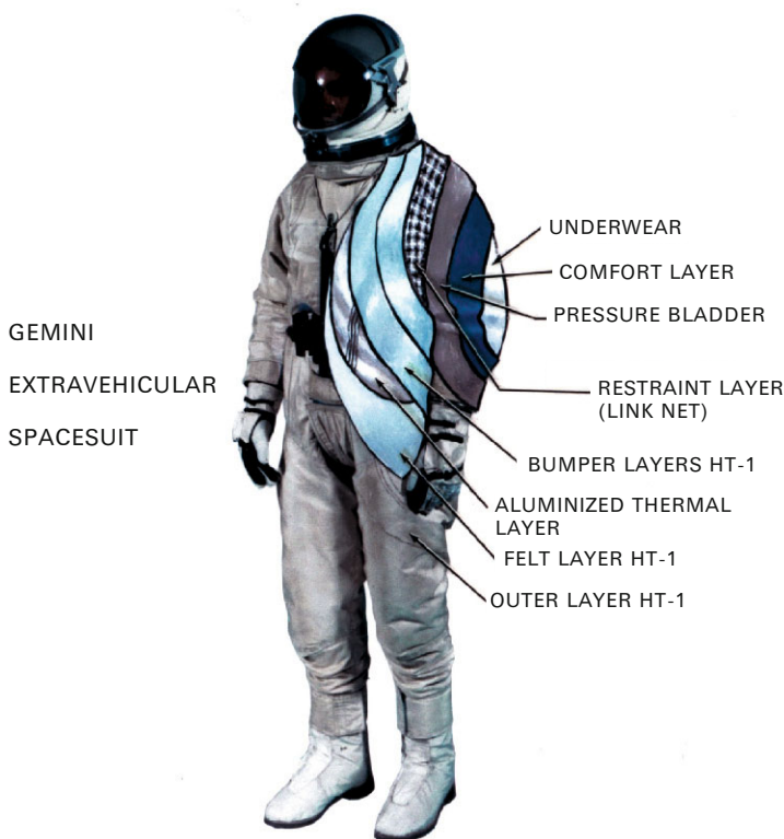
Figure 5.3.1. DCC Gemini IV suit materials (courtesy NASA).
