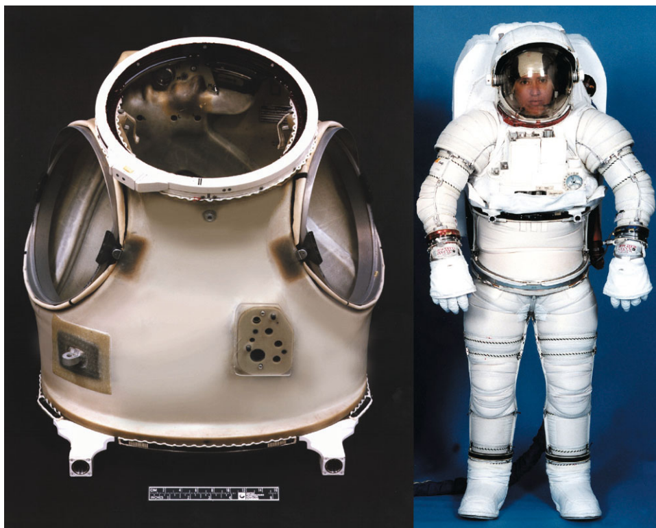
Figure 10.1.9. Pivoted HUT and baseline pressure suit (courtesy Hamilton Sundstrand).
