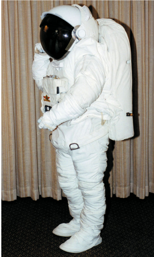
Figure 10.3.9. The Gilman & Gilliam small EMU prototype (courtesy Global Effects, North Hollywood, CA).
