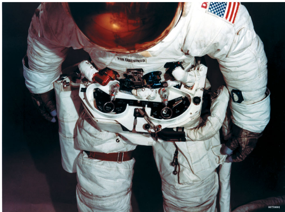
Figure 9.3.2. Skylab PCU attached to suit showing controls (courtesy NASA).
