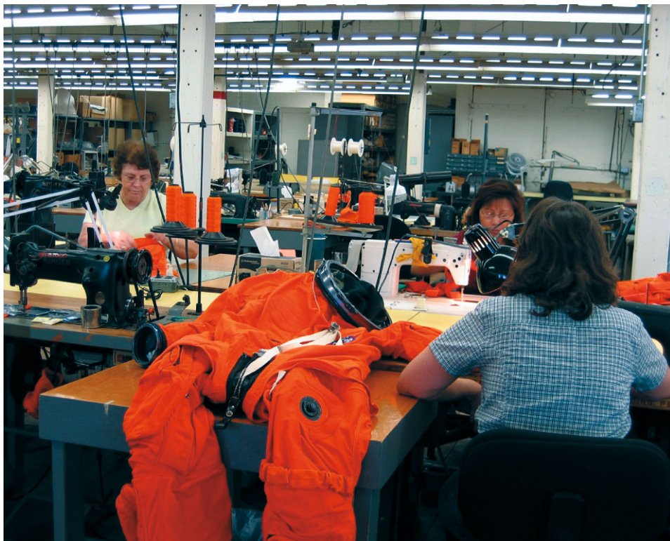
Figure 4.7.2. Shuttle ACES spacesuit manufacturing (courtesy David Clark Co.).
