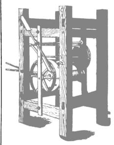
cscapement is bad. It is the old recoil, with iron scape wheel and anshor. As long as the oil is kept tresh and fluid, the clock keeps good time; but anything that decreases the force of the clock, causes it to gain very considerably, though Mr. Denison, in his work on clocks asys distinctly, the reverse is the case. Would putting a brass scape wheel, and suspending the pendulum by a very fine spring, remedy the defect? Can any of your readers tell me?
