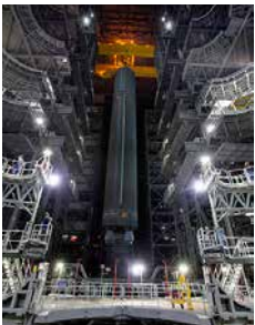
A crane lowers the Space Launch System Core Stage pathfinder into High Bay 3 in the Vehicle Assembly Building at NASA's Kennedy Space Center on Oct. 16, 2019. The pathfinder was used by Exploration Ground systems and its contractor, Jacobs, to practice offloading, moving and stacking maneuvers, using important ground support equipment to train employees and certify all the equipment works properly. Photo credit: NASA/Ben Smegelsky
