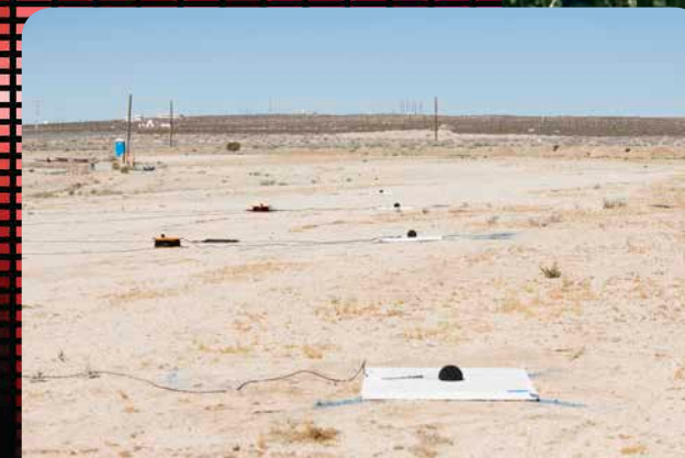
One of three microphone arrays positioned strategically along the ground at Edwards Air Force Base, California, sits ready to collect sound signatures from sonic booms created by a NASA F-18 during the SonicBAT flight series. Similar arrays will be set up near NASA's Kennedy Space Center to collect the sound signatures of booms that have traveled through atmospheric turbulence before reaching the ground. Photo credit: NASA/Lauren Hughes
