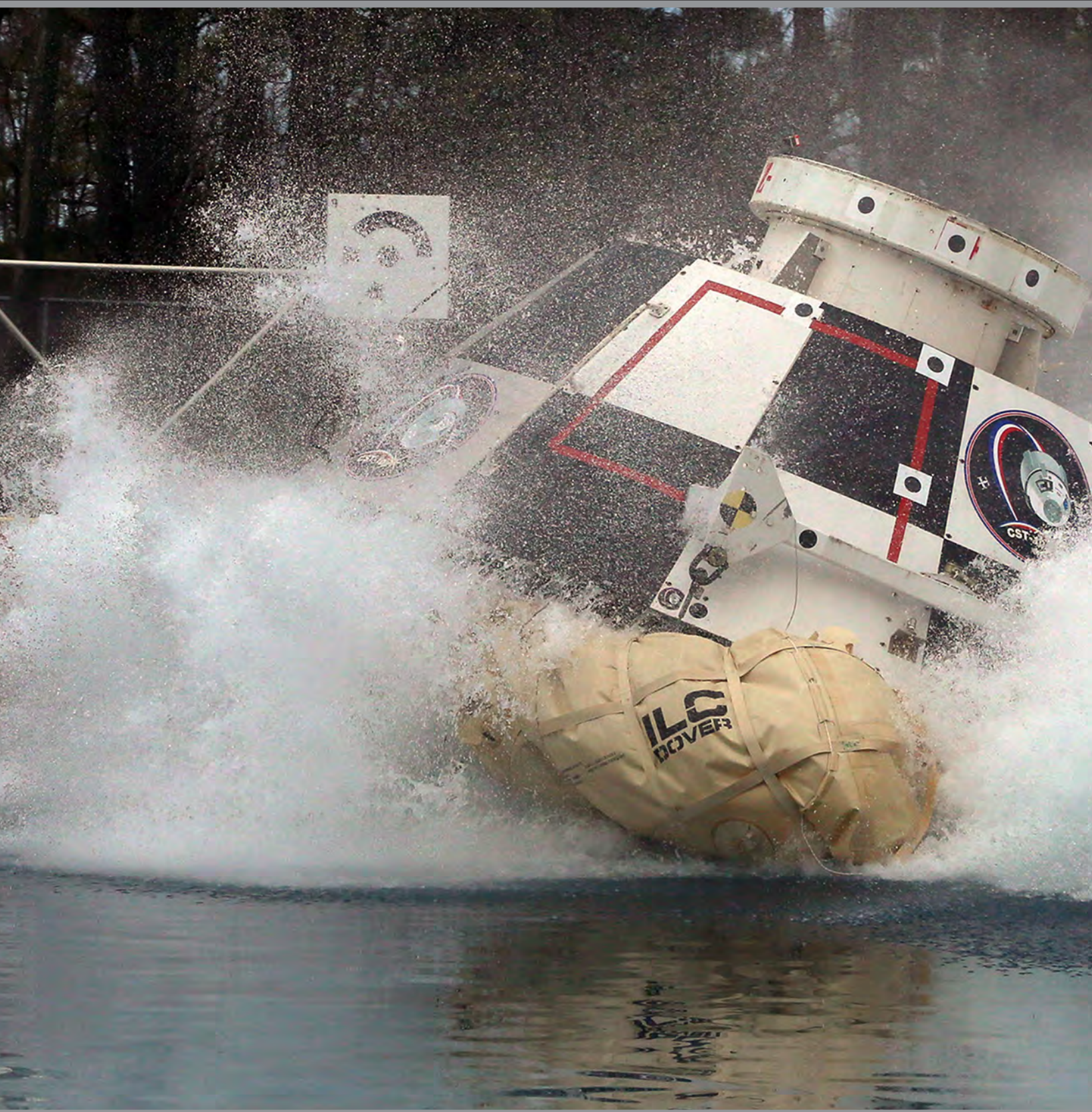
A mockup of Boeing's CST-100 Starliner splashes into a water tank at NASA's Langley Research Center in Virginia during landing system testing. Photo credit: NASA Langley
