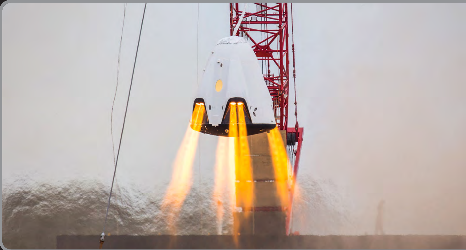
A full-size test article of a SpaceX Crew Dragon fires its eight SuperDraco engines in a development test of its ability to land with the accuracy of a helicopter using only the thrusters. Photo credit: SpaceX
