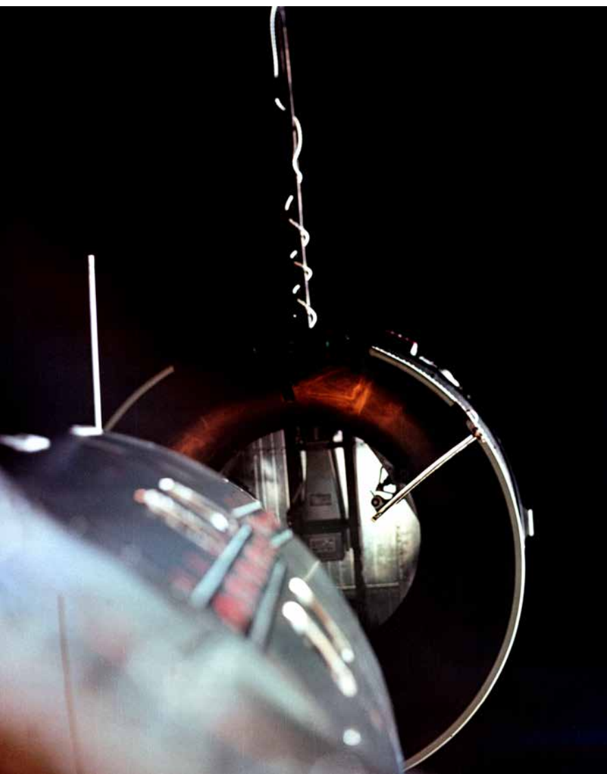
The nose of Gemini VIII approaches the docking collar of the Agena target vehicle as Neil Armstrong and David Scott complete the world’s first link-up between two spacecraft in orbit. Photo credit: NASA/David Scott
