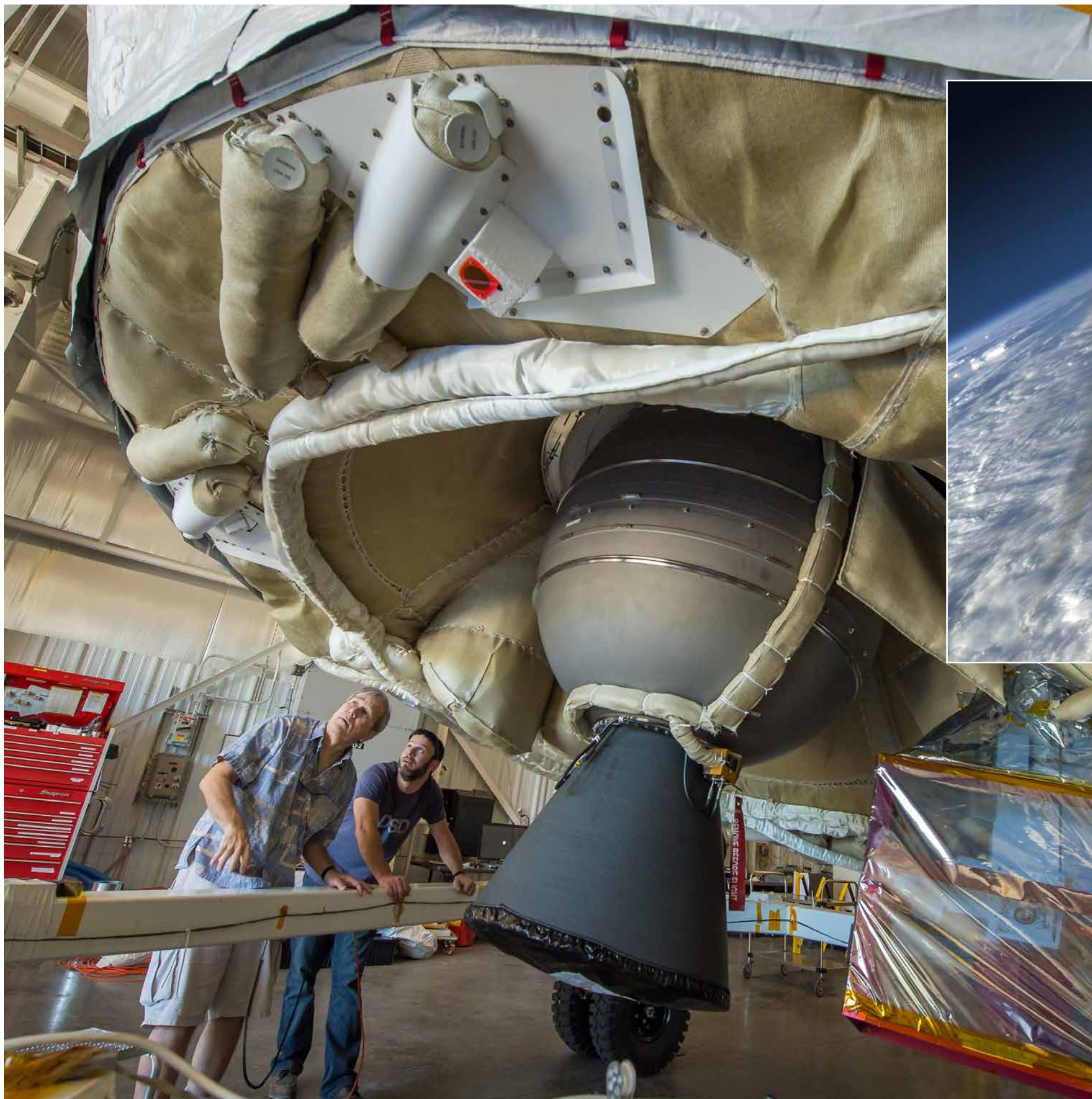
Above: This artist's concept shows the test vehicle for NASA's Low-Density Supersonic Decelerator, designed to test landing technologies for future Mars missions. A balloon lifts the vehicle to high altitudes, where a rocket takes it even higher, to the top of the stratosphere, at several times the speed of sound. Image credit: NASA
