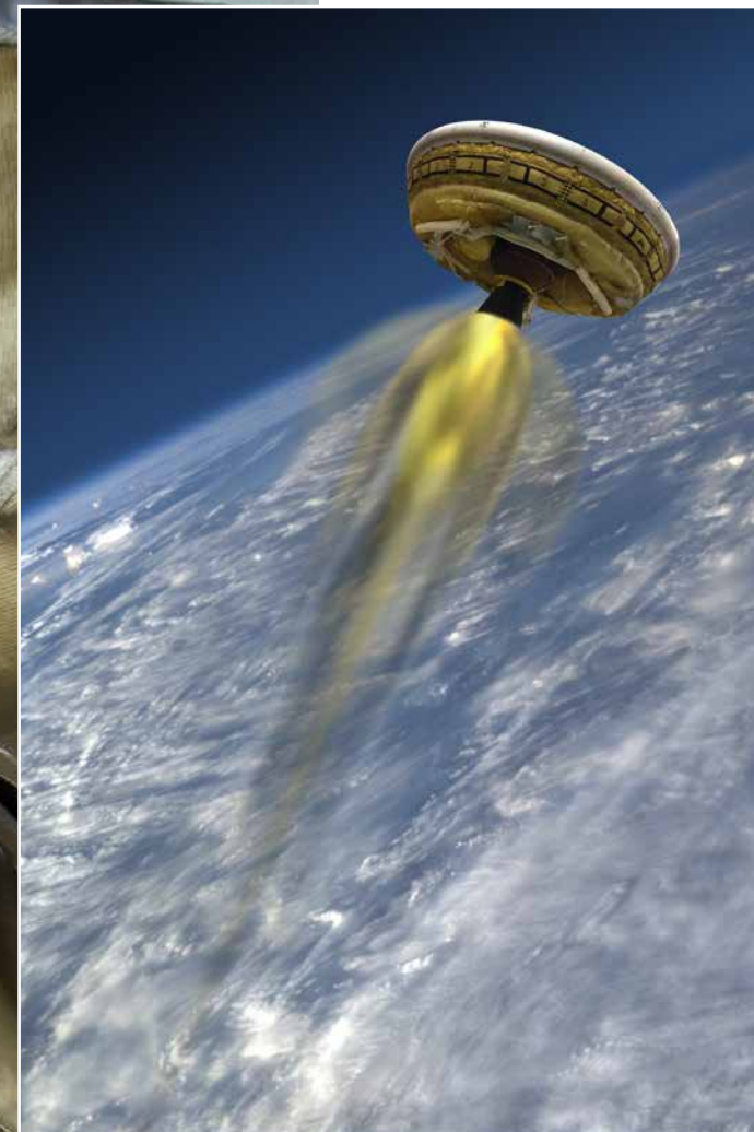
Above: This artist's concept shows the test vehicle for NASA's Low-Density Supersonic Decelerator, designed to test landing technologies for future Mars missions. A balloon lifts the vehicle to high altitudes, where a rocket takes it even higher, to the top of the stratosphere, at several times the speed of sound. Image credit: NASA
