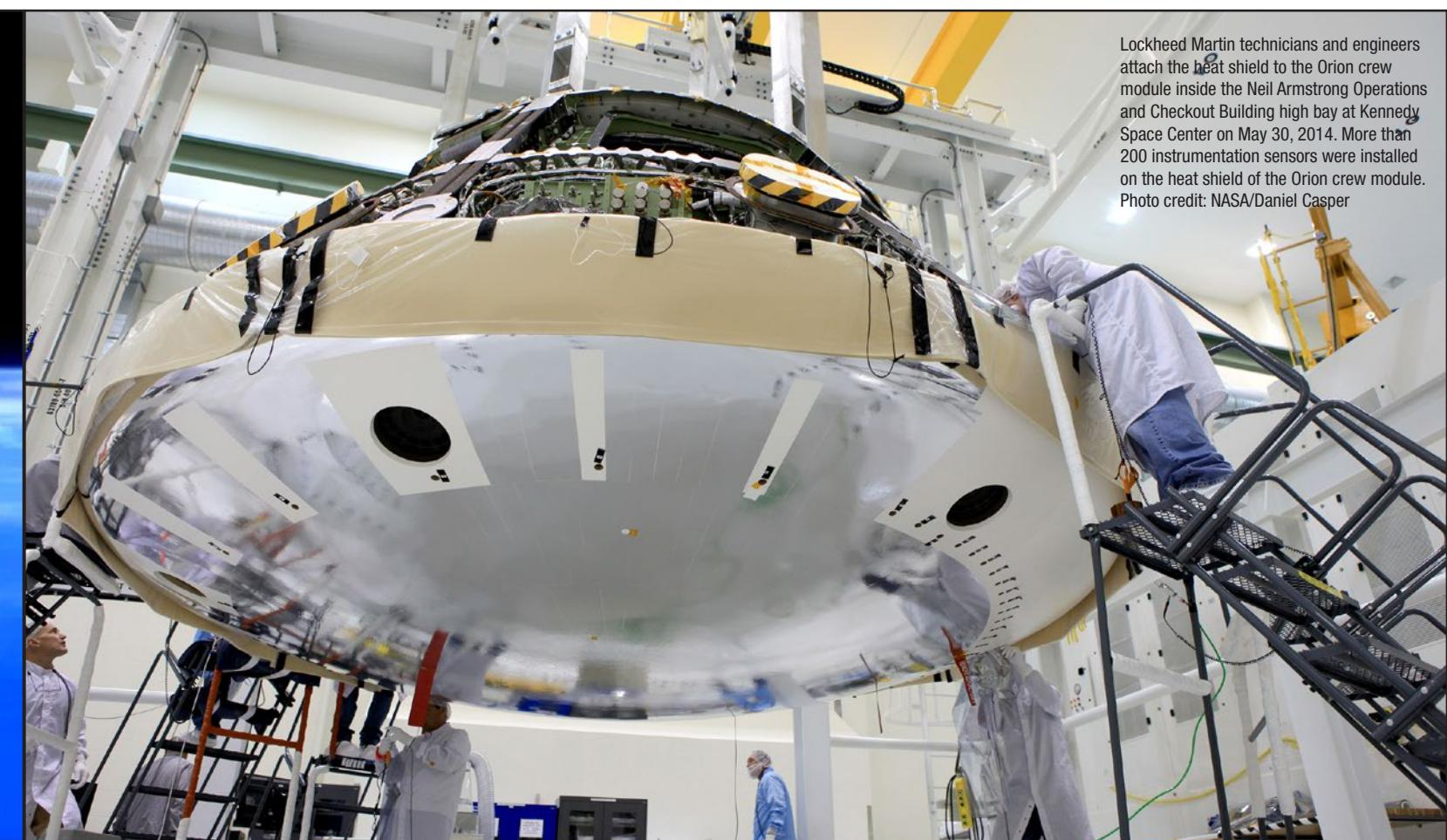
Lockheed Martin technicians and engineers attach the heat shield to the Orion crew module inside the Neil Armstrong Operations and Checkout Building high bay at Kennedy Space Center on May 30, 2014. More than 200 instrumentation sensors were installed on the heat shield of the Orion crew module. Photo credit: NASA/Daniel Casper
