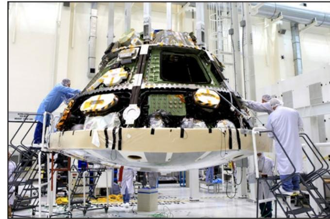
Inside the Operations and Checkout Building high bay May 30, 2014, Lockheed Martin technicians and engineers attach the heat shield to the Orion crew module for Exploration Flight Test-1. The mission will provide engineers with data about the heat shield's ability to protect Orion and its crews from the 4,000-degree heat of re-entry and an ocean splashdown following the spacecraft's 20,000-mph re-entry from space. Photo credit: NASA/Daniel Casper
