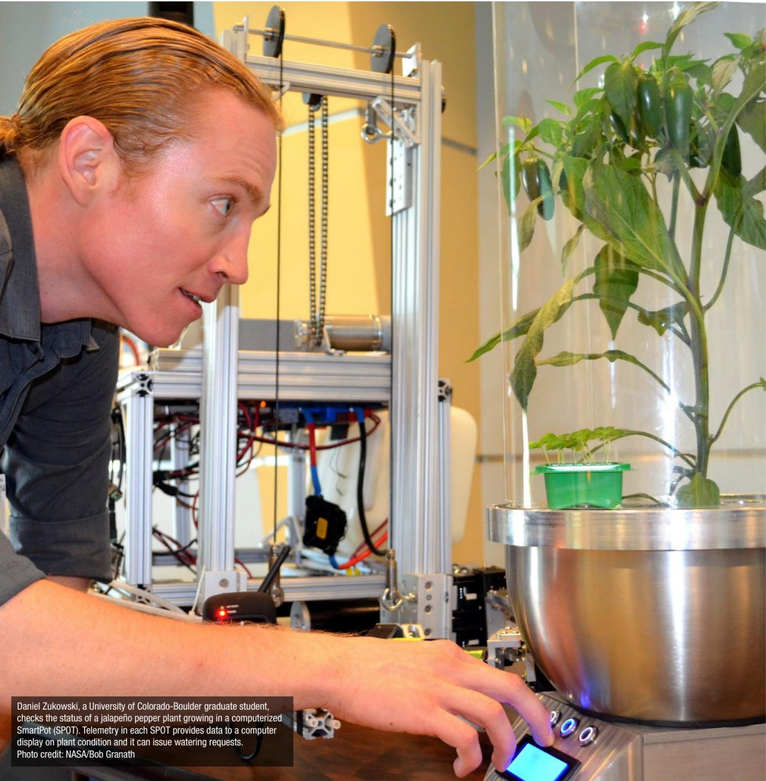
Daniel Zukowski, a University of Colorado-Boulder graduate student, checks the status of a jalapeño pepper plant growing in a computerized SmartPot (SPOT). Telemetry in each SPOT provides data to a computer display on plant condition and it can issue watering requests. Photo credit: NASA/Bob Granath
