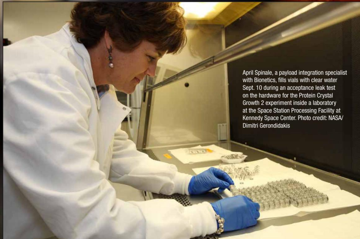
April Spinale, a payload integration specialist with Bionetics, fills vials with clear water Sept. 10 during an acceptance leak test on the hardware for the Protein Crystal Growth 2 experiment inside a laboratory at the Space Station Processing Facility at Kennedy Space Center. Photo credit: NASA/ Dimitri Gerondidakis
