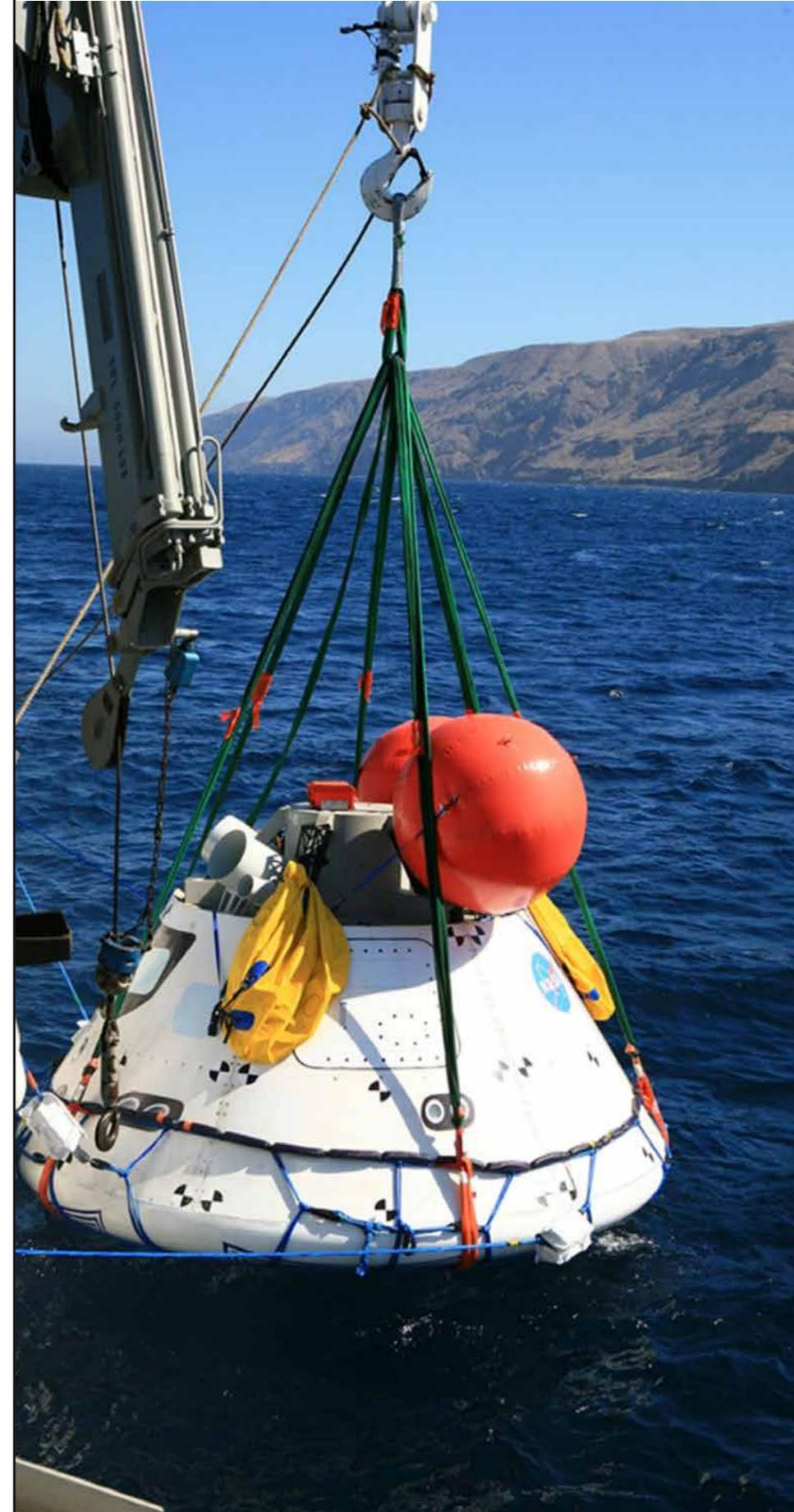
The Orion boilerplate test vehicle was lifted by stationary crane off the side of the USNS Salvor, a safeguard-class rescue and salvage ship, during Underway Recovery Test 4A in the Pacific Ocean on Sept. 14. Photo credit: NASA/Kim Shiflett
