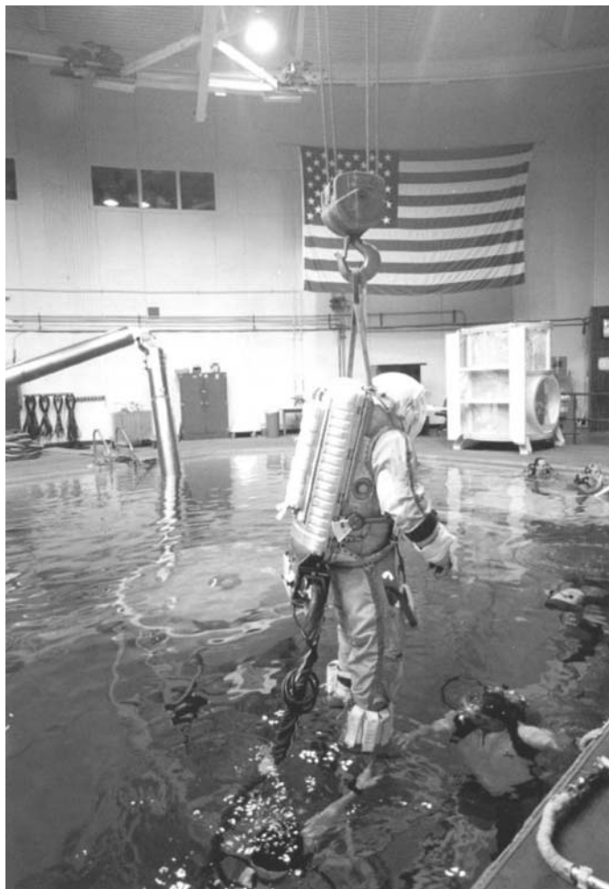
Mike Foale, wearing a specially weighted Orlan M training suit, is lowered into the WET-F at JSC for an evaluation of the Russian EVA pressure garment. (Courtesy NASA)
