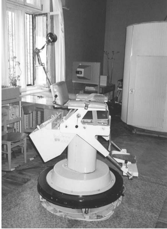
A rotating chair is used by the medical department to test and train cosmonauts for the effects of motion sickness
