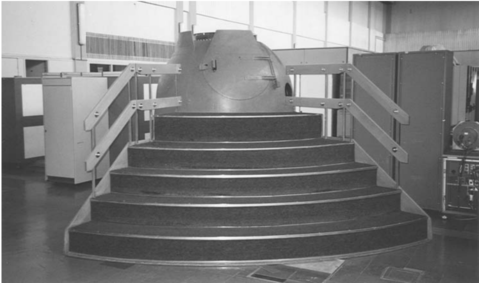
Pilot-732 is used for practicing approach and manual docking
