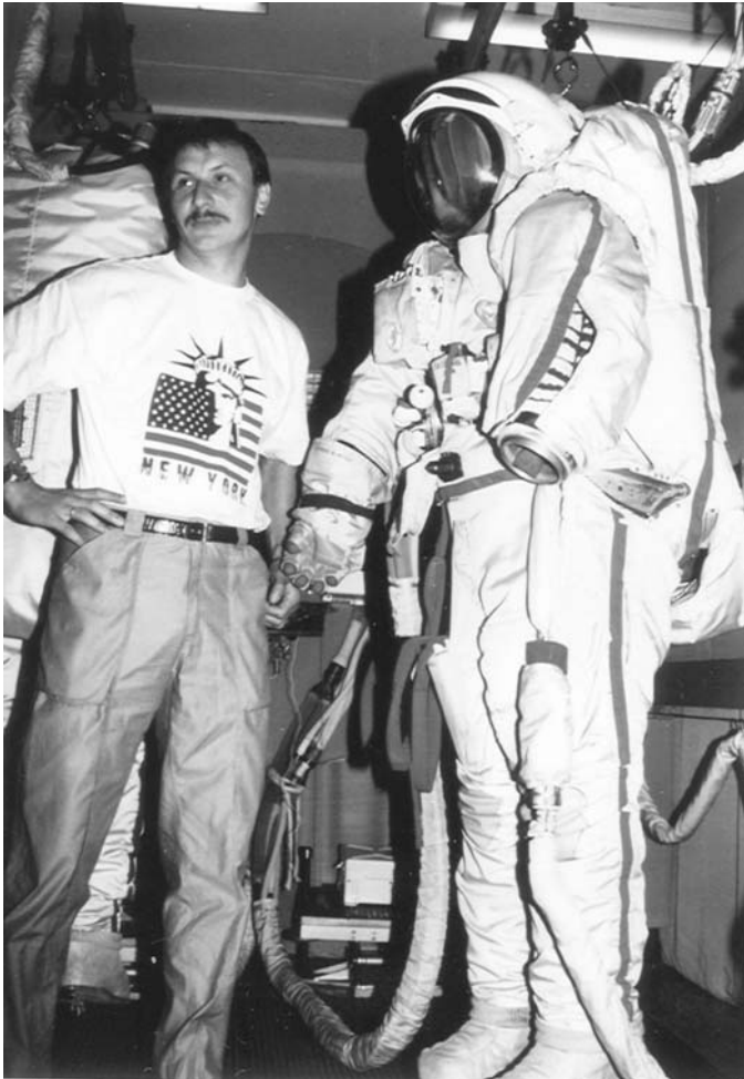
This is the Vykhod 1 facility which allows cosmonauts to get a feeling of weightlessness. It is located on the first floor of the Soyuz hall
