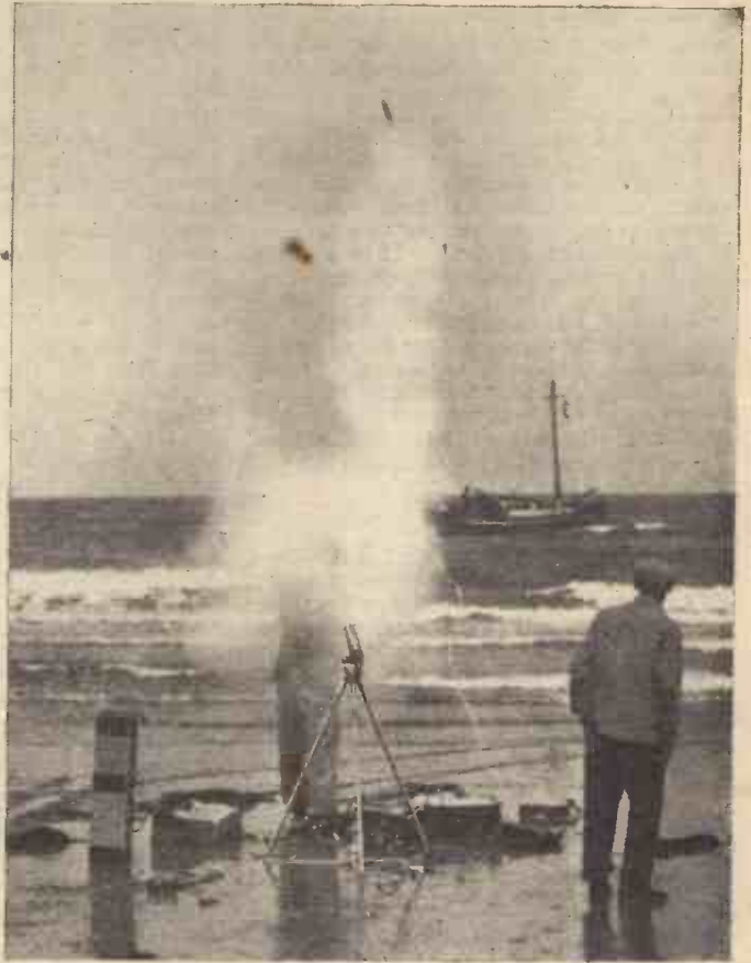
Operating No. 2 rocket hand-fired pistol. Range 250 yds.
