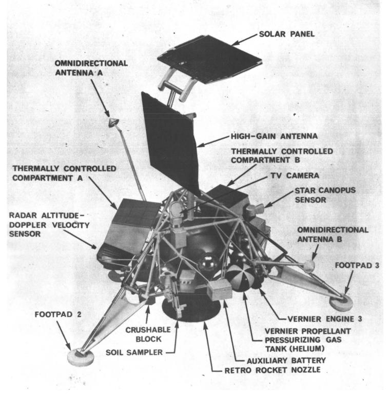
Two thermal compartments house sensitive electronic apparatus for which active thermal control is needed throughout the mission. The equipment in each compartment is mounted on a thermal tray that distributes heat throughout the compartment. An insulating blanket, consisting of 75 sheets of aluminized Mylar, is sandwiched between each compartment's inner shell and the outer protective cover. The tops of the compartments are covered by mirrored glass thermal radiators to dissipate heat.
