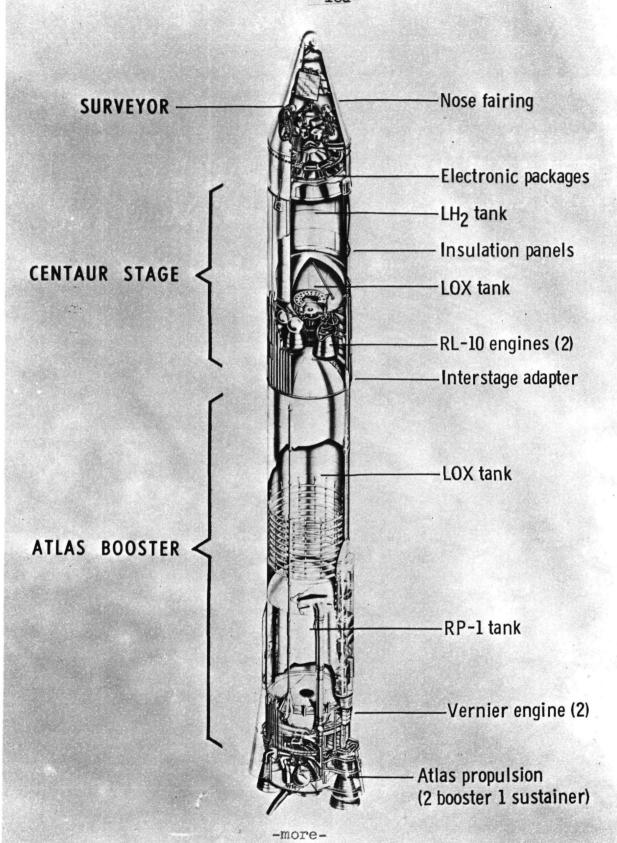
Major modifications to Atlas-Centaur to increase its payload capability include lengthening of the Atlas by four feet, which will increase total propellant capacity by some 20,000 pounds, and uprating of the Atlas booster and sustainer engines.
