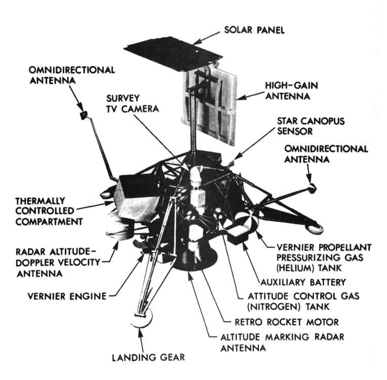
The equipment in each compartment is mounted on a thermal tray that distributes heat throughout the compartment. An insulating blanket of 75 sheets of aluminized Mylar is sandwiched between each compartment's inner shell and the outer protective cover. The compartment tops are covered by mirrored glass to help radiate the heat.
