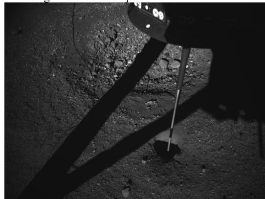
Figure 4: Image acquired from the SCALPSS short focal length camera number 3 (SFL3) showing the LISTER drill and hole (right of center), a wire connected to one of the deployed LMS electrodes (left of center), and a view of the surface rocks and regolith size distribution [image provided by C. Nguyen/NASA LaRC].
