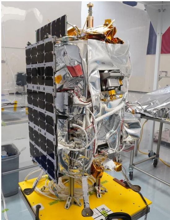
Figure 2: IM hopper. Approximately 70 cm tall, and capable of flying 8 kg of payload several kilometres.
