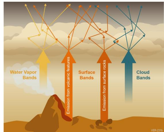
**Figure 1** VEM maps surface rock type and search for evidence of volcanic activity by its thermal signature and by an enhancement of water vapor near the surface. A dedicated set of bands is used to correct for the effect of clouds.
