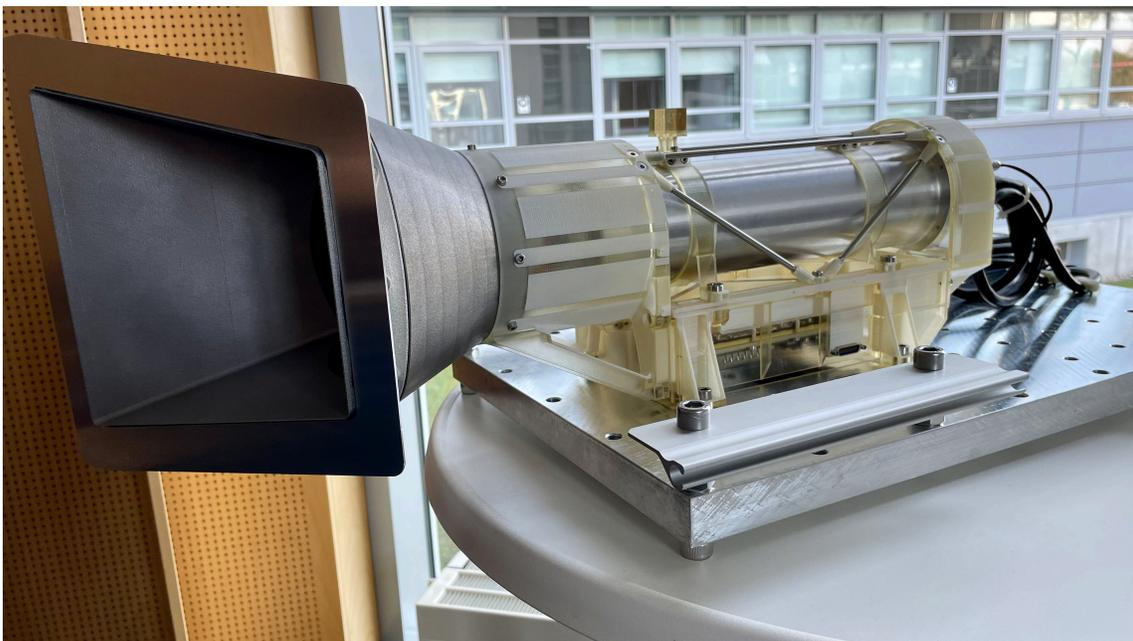
**Figure 2** VEM prototype with flight like optics, flight like baffle (without coating), flight-like detector and updated mechanical design including stiffener - housing is replaced by representative 3D print for visualization
