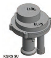
Fig. 1 Drawing of KPLO GRS sensors. Adapted from [3].
