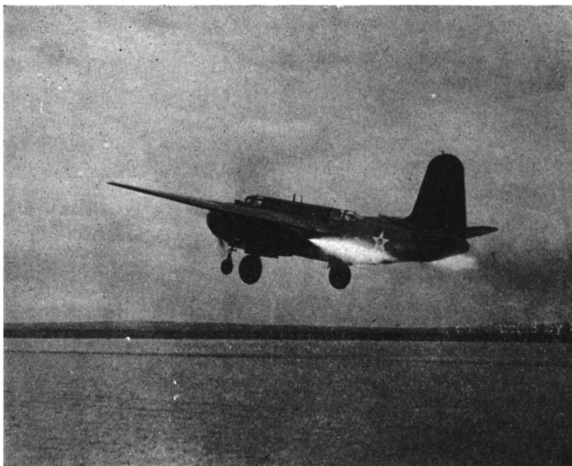
A-20A Take-off assisted by two 1000 pound thrust, 25 second duration liquid motors.
