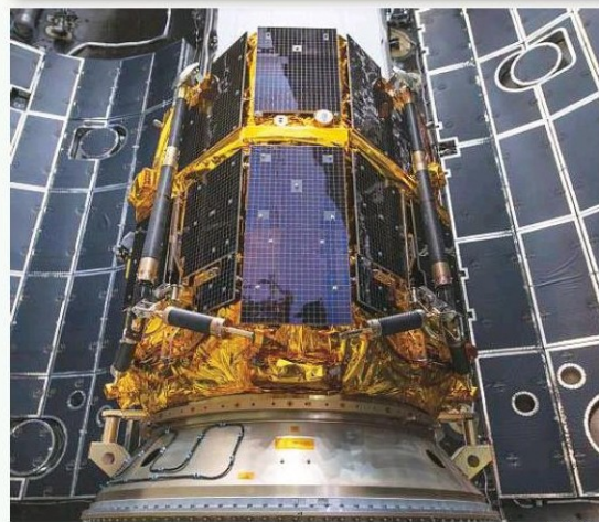
Hakuto-R, Hakuto-R M1, which means 'white rabbit' in Japanese, will carry the Rashid Rover to its destination.
