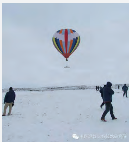
The balloon lifting the test rocket stage for a recovery test. (credit: WeChat/CALT)
