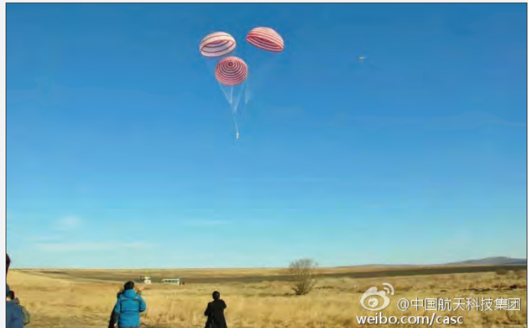
The parachutes developed for the new generation manned space vehicle in drop testing. (credit: Weibo/CASC)
