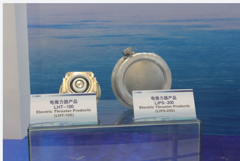
The LHT-100 and LIPS-200 electric thrusters (credit: Chinese Internet)
