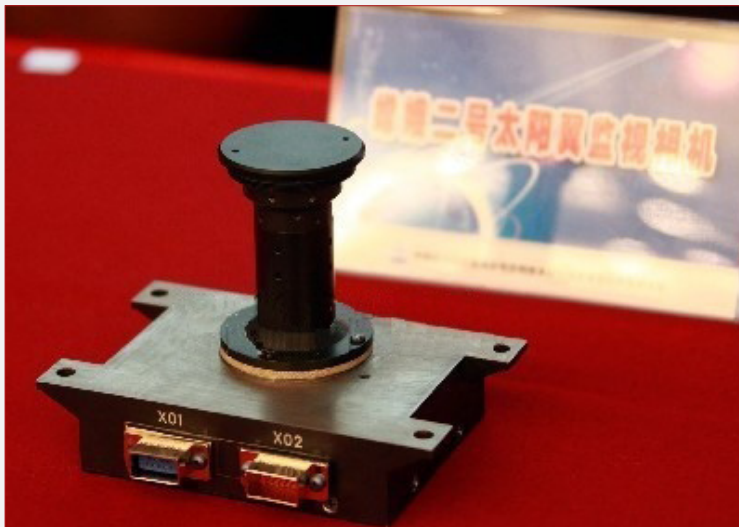
The solar wing surveillance camera that played a key role in the Toutatis flyby (credit: Chinese Internet)
